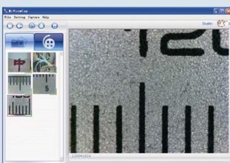
5. Now the software is ready to take new images with the calibrated magnification at this focus point (Don't adjust the “Focus & Magnification adjustment wheel”), thus the measurement for these captured images after calibration will be very accurate and the error rate of measurement is under 3%.
