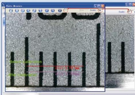
4. The software will automatically calibrate the scale of magnification and will show the calibrated scale of magnification at the right-hand box of calibration button, and also automatically adjust the scale of main program on this focus point.
