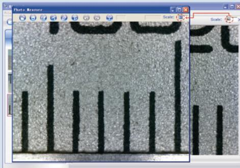
2. Now double click to open the image of the measurement calibration standard (图3), and the scale of magnification will be automatically loaded for measuring.
